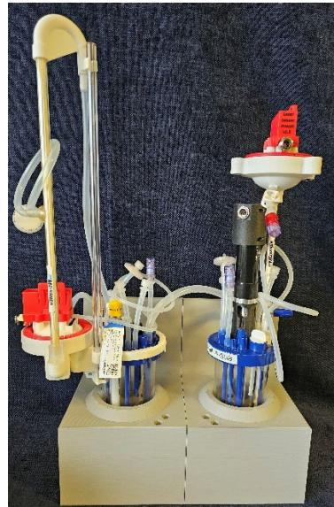
*LASER sensor mounted in the red bracket above the dome of the Thalia TM80 pump. The P-SUBmerged ATF SUB is driven by DASbox and supplied with complete hose set for easy installation.*
