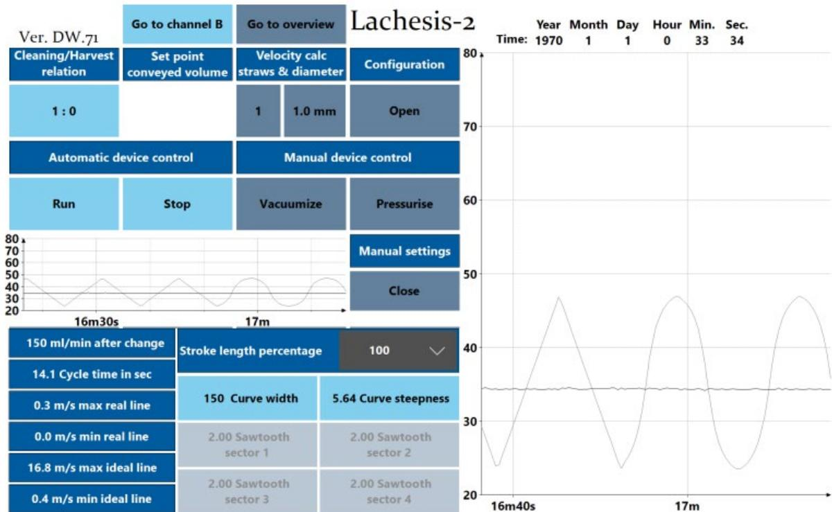
*Lachesis screen with adjustment panel open, configuration panel closed, manual setting picked and sinus curve running*
