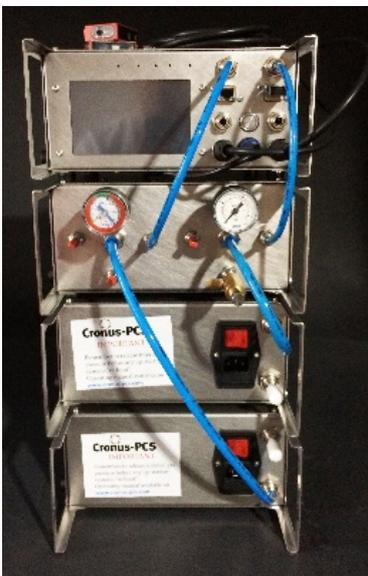
*Refer to section "2. Device Overview" and be sure you connect vacuum to the left and pressurizes air to the right.*
