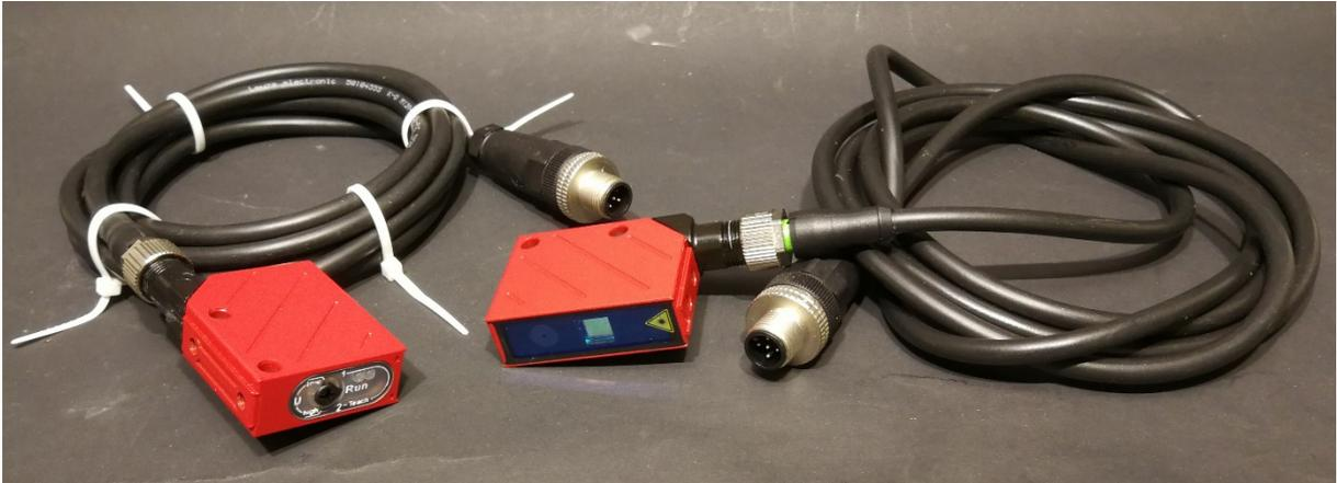
Two identical Leuze Laser sensor's shown with 1,5 meter wire and M12 connectors.
