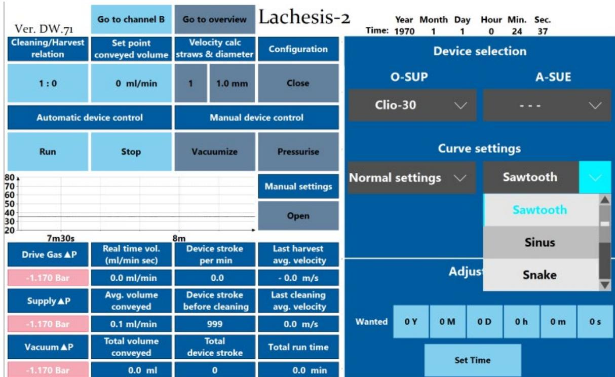
Graphical-User-Interphase (GUI) for Lachesis drive unit operate with different colours. Light red is warning info from pressure sensors. Dark blue lower rectangle is Apollon PLC information.
