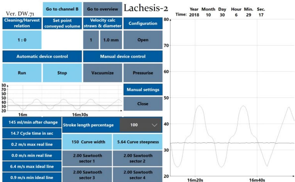
*Lachesis screen with adjustment panel open, configuration panel closed, manual setting picked and sawtooth\_4 curve running*
