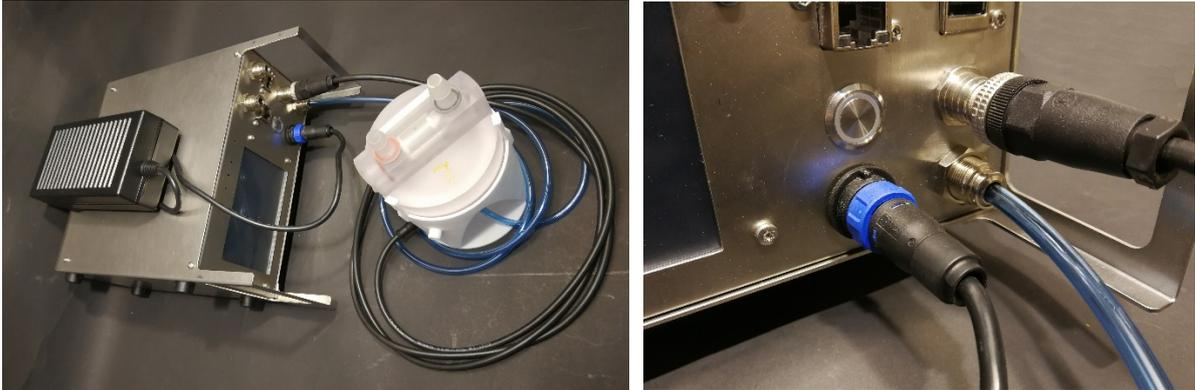
*Focus with these photos is how SUP and Power Supply (PS) is connected. PS connection is simple with the round bright blue finger nut on the black Buccaneer cable connector. Drive gas is via the transparent blue soft polyurethane hose. Laser sensor input via the black M12 cable connector.*
