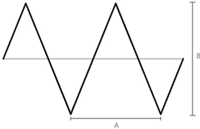
Sawtooth curve, A is equal to one pump cycle and B is equal to stroke length
