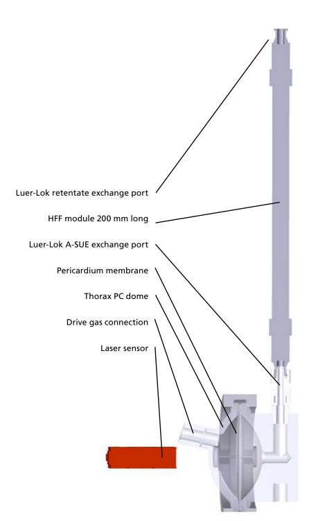
The A-SUE is arranged inside a Polycarbonate housing with no liquid valves. The A-SUE exchange liquid forth and back.
