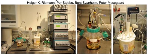
Set-up on DasGip with batch in traditional glass/steel STR on stirrer table 1 and perfusion SUB on stirrer table 2
